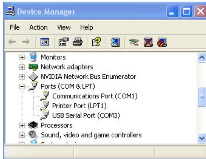
In the case above the serial port is allocated to serial port COM3 however may vary depending on pre-existing com port hardware and virtual drivers loaded for other applications. The device manager list can be located by selecting the Start>Control Panel>System Menu and then selecting the Hardware>Device tabs.
